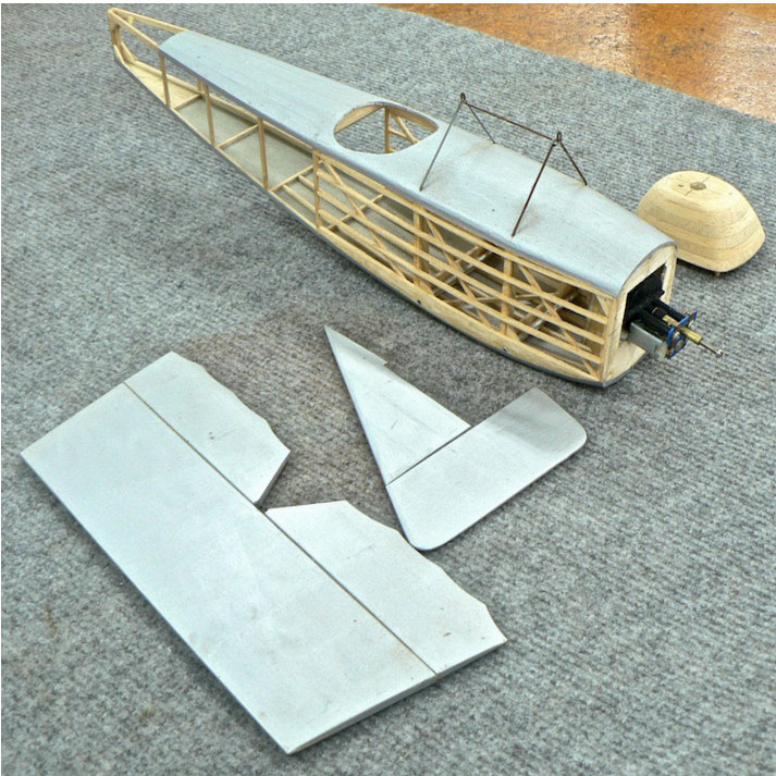
Above: The fuselage of Mike Mulholland's re-engineered Airsail PC-9 is much lighter than the original.
