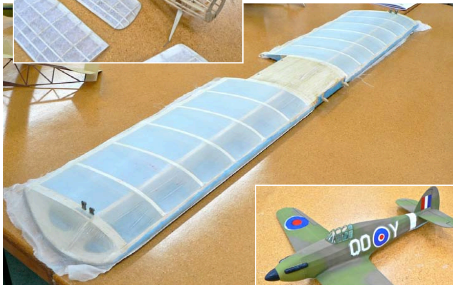
Above: Evidence of Charles Warren's first foray into silk over mylar covering - definitely a success.
