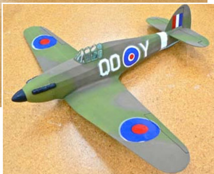
Above: Evidence of Charles Warren's first foray into silk over mylar covering - definitely a success.
